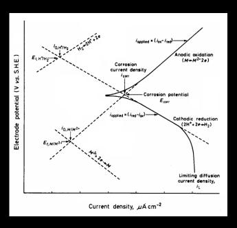
At any time: TOTAL RATE OF OXIDATION = TOTAL RATE OF REDUCTION
